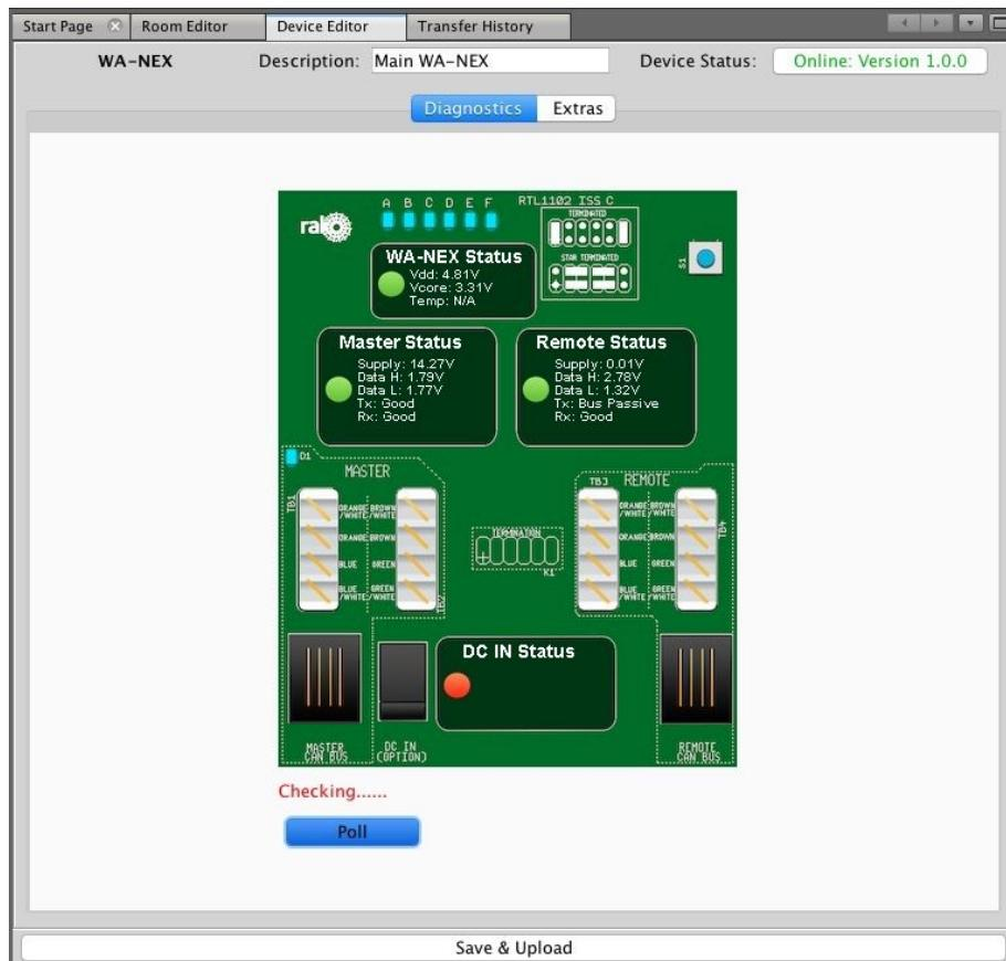
Pressing "Poll" will run a diagnostic check on both sides of the system. If there is a problem such as "Remote CAN Voltage too low" or "Short on Master Data side" it will appear to the right of the screen in Rasoft Pro. In most cases an advised course of action will also be given.
