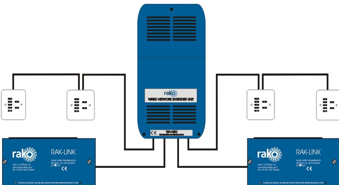
A system with approximately two fully populated RAK-Stars will be approaching the 3000m limit in a typical installation. Obviously this can vary dramatically depending on the nature of the installation and resulting routes taken by the cables.
