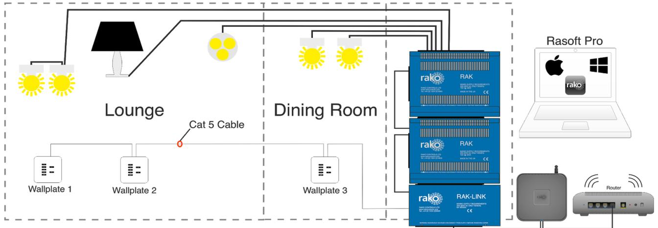
The RAK-LINK is used to integrate the RAK(s) into the Rako Wired Network and can support a total of 32 circuits. For example 4 RAK8s or 3 RAK8s and 2 RAK4s.
