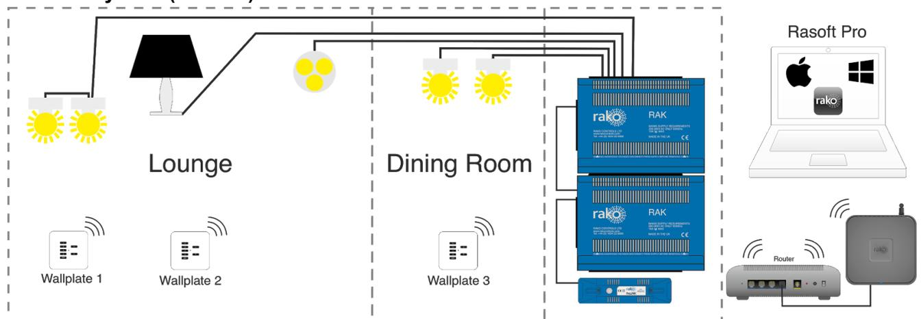
The RxLINK is used to integrate the RAK(s) into the wireless system and can support a total of 16 circuits. For example two RAK8s or one RAK8 and two RAK4s.
