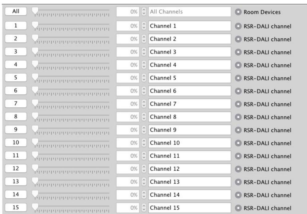
The RSR-DALI is a multi-channel device and will occupy the entire room. By default Short Address 0 will be addressed to Channel 1 in the Rako Room, DALI Short Address 1 to Channel 2 and so on for all 15 Channels.
