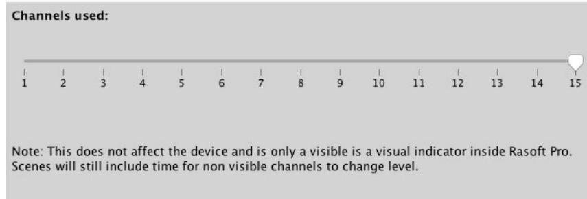
Slide the “channels used” slider to match the number of Channels required by the RSR-DALI and the remaining channels are freed up to be used by other devices.
