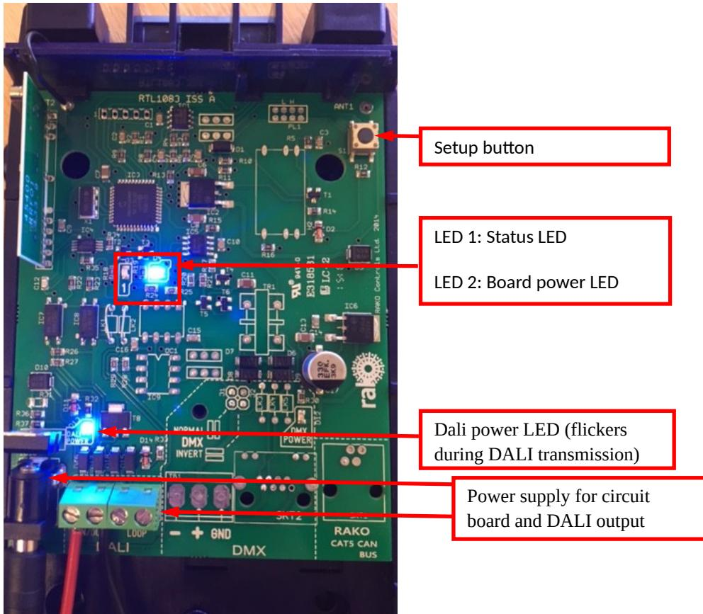
The RSR-DALI requires 18V DC, a suitable power supply attached to a 13A plug is provided with the product. When successful powered up LED 2: the “Power LED” will illuminate.
