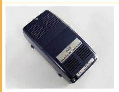
The WAVFR is fitted with a 10 way set of screw terminals for signal input and an additional 3 way connector for Common inputs. The WAVFR is configured in Rasoft and signal inputs can trigger lighting scenes or actions in a similar fashion to button presses on a wallpanel.
