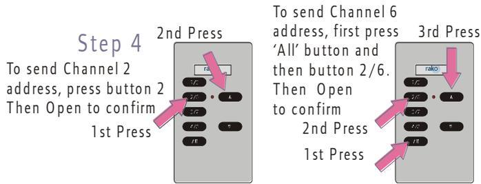
**Setting an address from a single channel controller**
