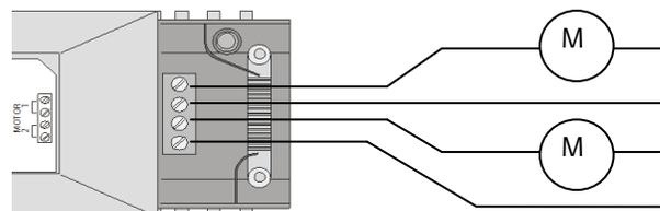
Once the supply and load cables are connected ensure that the terminal covers are replaced and securely fastened, clamping the cable correctly before powering the unit.
