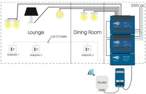
The RAKLink is used to integrate the RAK8(s) into the Rako Wired Network and can support a total of 32 circuits. For example 4 RAK8s or 3 RAK8s and 2 RAK4s.
