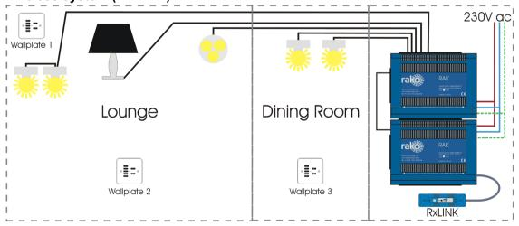
The RX-Link is used to integrate the RAK8(s) into the wireless system and can support a total of 16 circuits. For example two RAK8s or one RAK8 and two RAK4s.
