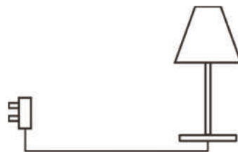
Incorporate a free standing lamp by wiring a Rako dimmer into a flex.
