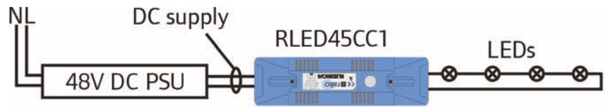
Single channel constant current 45W LED dimmer
