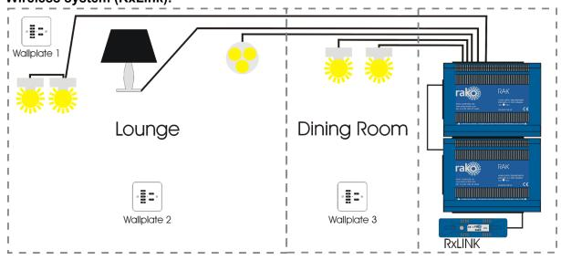
The RxLINK is used to integrate the RAK(s) into the wireless system and can support a total of 16 circuits. For example two RAK8s or one RAK8 and two RAK4s.
