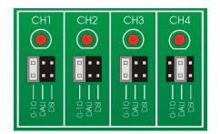
The digital output type is set by using the jumpers on the circuit board. Output type can be set separately for each channel of the RAK4-F. If all jumpers are removed then the RAK4-F will default to 0-10V mode.
