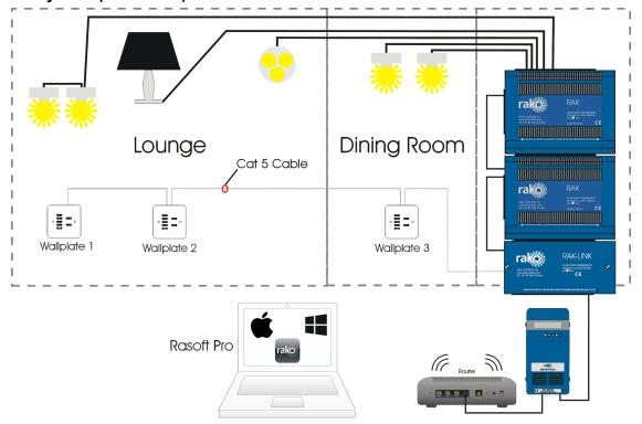
The RAK-LINK is used to integrate the RAK(s) into the Rako Wired Network and can support a total of 32 circuits. For example 4 RAK8s or 3 RAK8s and 2 RAK4s.
