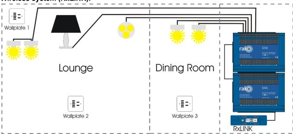
The RxLINK is used to integrate the RAK(s) into the wireless system and can support a total of 16 circuits. For example two RAK8s or one RAK8 and two RAK4s.
