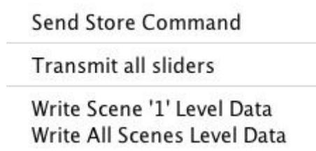
These extra options allow scenes to be transmitted without the need to individually reset every slider for every channel. This is particularly useful when a dimmer has been swapped and the scenes need to be reuploaded to match those in the removed dimmer.
