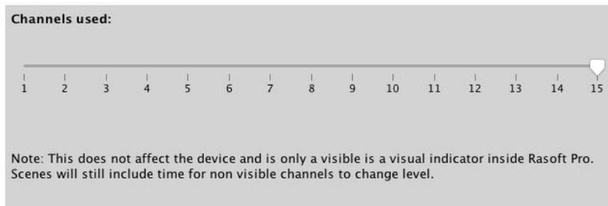
Slide the “channels used” slider to match the number of Channels required by the WSR-DLI and the remaining channels are freed up to be used by other devices.
