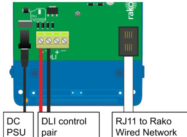
The WSR-DLI must be connected to the Rako wired system by the RJ11 port either plugged directly to RAK-LINK or RAK-STAR or punched down to the CAT5 cable via a WP-CONC. The WSR-DLI requires 18V DC, a suitable power supply attached to a 13A plug is provided with the product. When successful powered up LED 2: the “Power LED” will illuminate.
