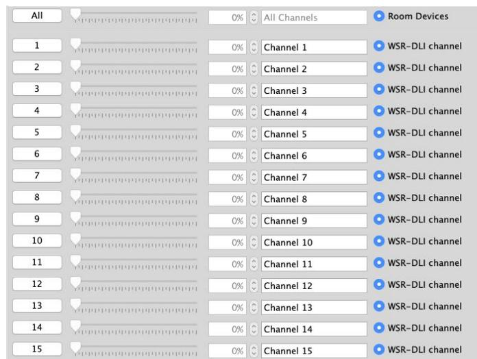
The WSR-DLI is a multi-channel device and will occupy the entire room. By default Short Address 0 will be addressed to Channel 1 in the Rako Room, DLI Short Address 1 to Channel 2 and so on for all 15 Channels.
