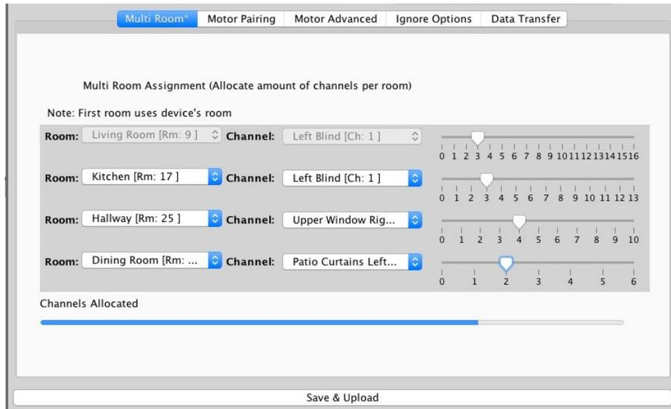
For example in the image above there are 3 channels in the Living Room, 3 in the Kitchen, 4 in the Hallway and 2 in the Dining Room. The blue bar along the bottom indicates the number of channels allocated of the total of 15.
