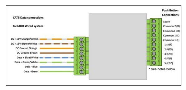
The WCM-D is wired into 2 pluggable sets of terminals. The 8 way terminal block connects to the Rako wired network formed of cat5/cat6 cable with cable allocations as set out above.
