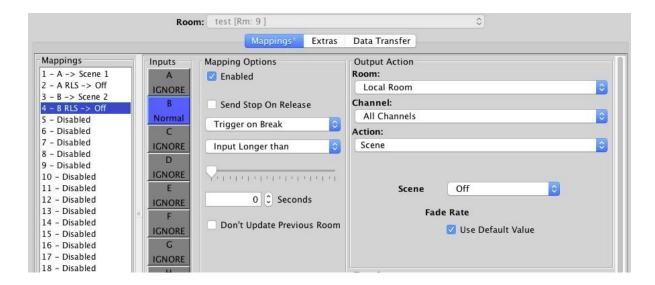
Above is an example of how a two way latching switch would be programmed when wired in to inputs A and B of a WCM-D.
