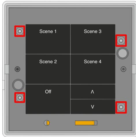
These must not be adjusted. Adjusting these may damage WK-MOD-xxx-x
