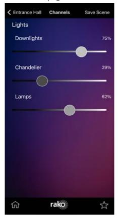
The lighting circuits that have been associated with this room and uploaded to the HUB will be displayed here. The light levels can be manually set from this page by sliding the slider to the desired lighting level. In this way one off "scenes" can be created for special events or parties where lighting moods not usually assigned to a button are required.
