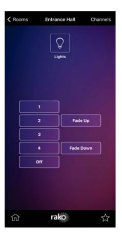
A room to control curtains and blinds will have "Open", "Stop" and "Close" options whereas a lighting room will have a number of scene buttons, fade up, fade down and off (both displayed above).
