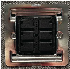
The keypad is orientated with the LED light holes at the top outer corner of each button.
