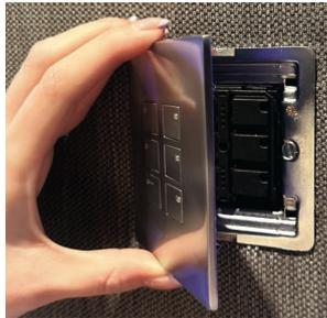
The front plate is connected by four clips in the corners of the plate
