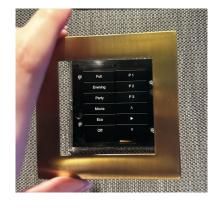
Care should be taken when removing the HS-MOD surround. To remove the surround, pull away from the wall squarely towards the installer.
