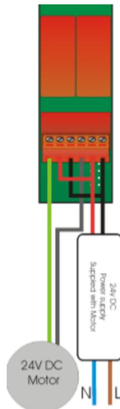
Contact closure blind wiring diagram:
