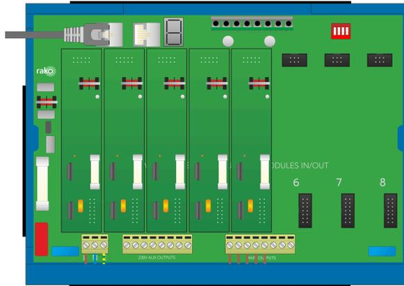
Insert the RJ45 cable from the RAK-LINK/RxLINK into the port on the RAK and from there another RJ45 cable to each RAK in the "stack".
