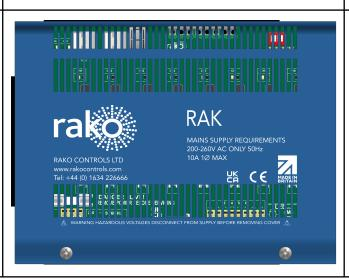
Screw down the circuit board to secure it to the case and fit the lid to complete the installation.
