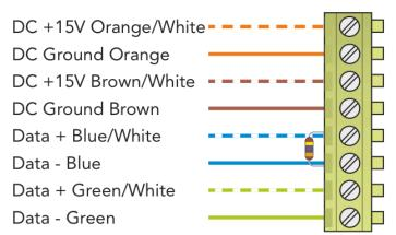
When the WCM-D is in the end of line position and not connected to a RAK-STAR a 120 Ohm resistor termination is required. This is provided with the WCM-D. The resistor is placed between the Blue and the Blue/White inputs.
