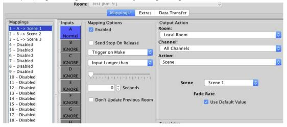
Above is an example of how a three way momentary switch would be programmed when wired into inputs A, B, and C of a WCM-D.
