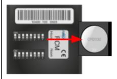
4. Remove the old batteries, making note of their orientation and type.,
