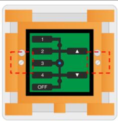
3. Slide out the battery tray, and take note of the tray and battery orientation.
