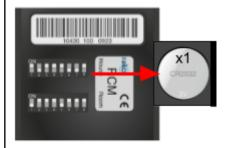
3. Remove the old batteries, making note of their orientation and type.,
