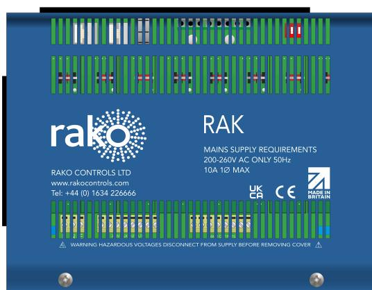
The RAK8-MB is a modular eight-slot motherboard designed to house dimming and switching cards. The modular design enables the RAK8-MB to have fully customisable outputs via the interchangeable RAK8-MB cards.
